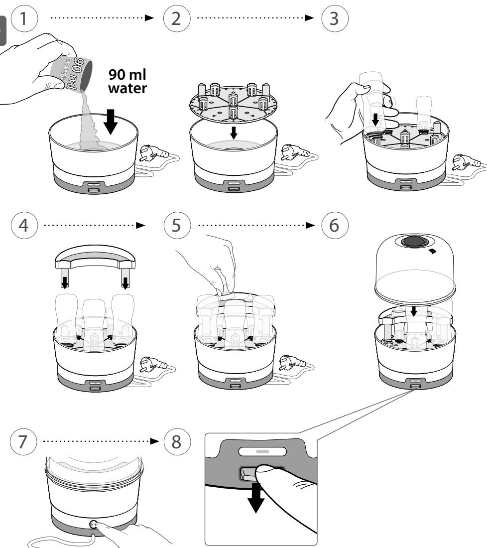
**Please rinse all parts to be disinfected before starting the process and remove any food residue. Position the bottles and accessories in such a way that they are not touching the walls or cover.**
